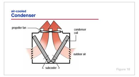
In a typical **air-cooled condenser**, propeller-type fans are used to draw outdoor air over a fin-tube heat transfer surface. The hot, high-pressure refrigerant vapor flows through the tubes as heat is transferred to the cooler outdoor air. The resulting reduction in the heat content of the refrigerant vapor causes it to condense into liquid. Within the final few lengths of condenser tubing the condensed liquid refrigerant is subcooled.
